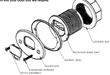
'Sealant is not generally required in installing the Tallon<sup>TM</sup> Socket system but in certain circumstances it may be desirable to use an appropriate marine sealant
